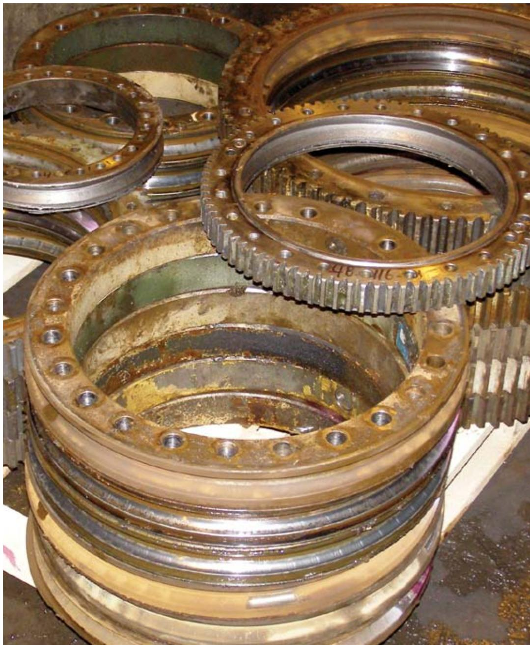
Corrosion is the natural enemy of a rolling element bearing, and a sneaky enemy at that. When chemical reactions from moisture, vapors and acids attack bearing surfaces, the damage they cause often isn't apparent until it's too late. Fortunately, there are many things you can do at the design stage to protect your bearing from these sneak attacks.
